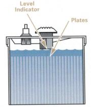
Maintain electrolyte level from at least 1/2-inch (13 mm) above plates to 1/4-inch (6 mm) below level indicator.
