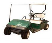
Single Seat Back Metal Body Front Black Plastic Nose Cap DCS & Series or 295cc 4 cycle 54" Top With Handles
